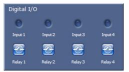
The alarm icons **Input 1** to **Input 4** are for information purposes and indicate the status of an alarm input: When an alarm is triggered, the corresponding icon lights up blue. The unit's configuration determines whether the alarm is displayed, as well as additional details (see *Section 5.15 Advanced Mode: LIVEPAGE Functions, page 42*).
